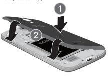
2. Press along the edge of the back cover (3) until you have a secure seal
